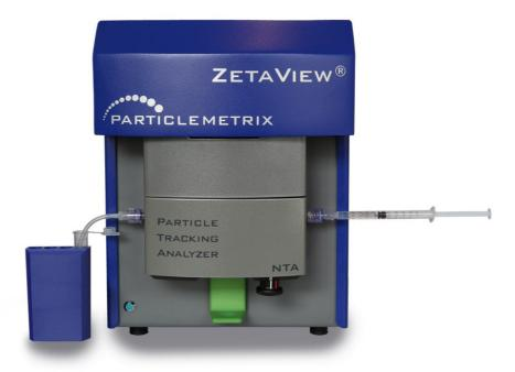
**Figure 2:** ZetaView set-up with corresponding NTA-cell assembly. The sample is injected via a syringe on the right and collected on the left using an Eppendorf tube.
