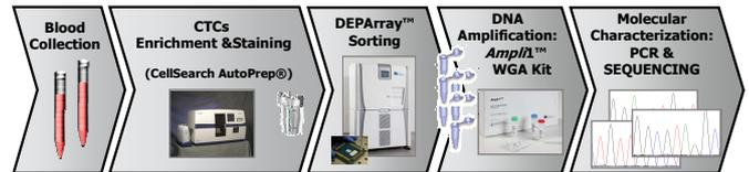
Fig.1 Sketch of workflow based on the DEPArray™ Rare Cell Isolation Technology for CTCs separation and molecular characterization from blood samples enriched with Veridex CellSearch® CTC Kit.
